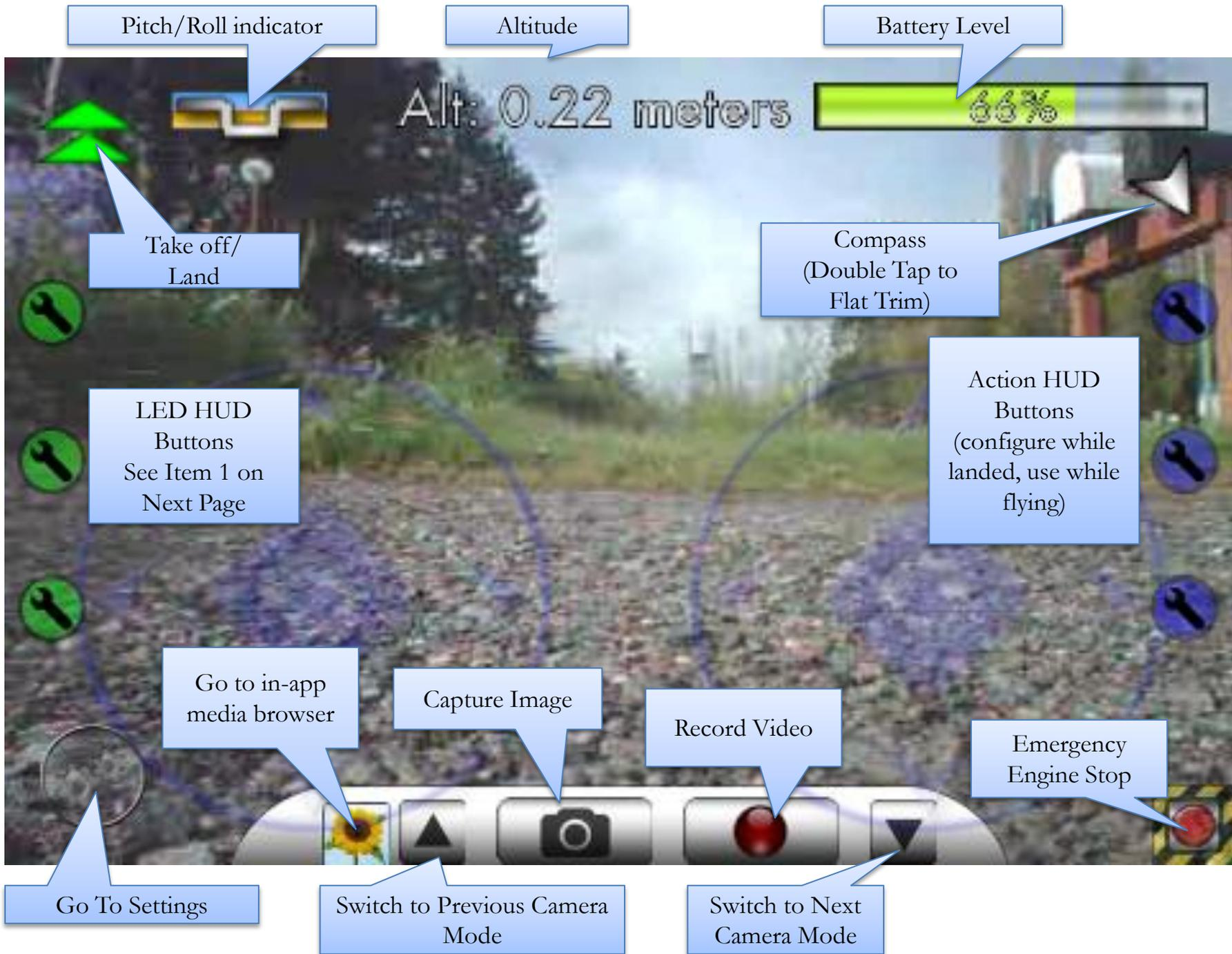
1. LED HUD Buttons – The LED HUD Buttons on the left side of the screen are configured when landing as indicated by the wrench icon. Tap the button while landed to select the LED flash pattern that you would like displayed on the AR.Drone. When the AR.Drone is flying, you can push these buttons to cause the LED Pattern you selected to show on the AR.Drone.
